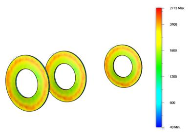
Figure 12: FEA on Motor Mount Centering Rings (von Mises Stress)
