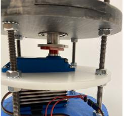
Figure 25: Servo Motor and Aluminum Hub Attachment
