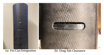
Figure 29: Integrated Air Braking System Tabs
