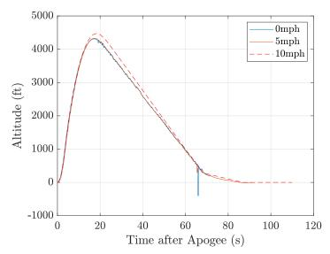
Figure 94: Simulation compared to payload verification flight
