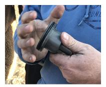
Figure 103: The O-ring around the forward enclosure
