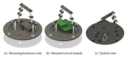
**Figure 51:** Renderings of fully assembled telemetry retention system. First picture demonstrates the retention system without electronics, second demonstrates retention system with mockup circuit boards, third picture shows eyebolt mounted to aft side of retention bulkhead.
