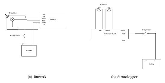
Figure 42: Altimeter Wiring Diagrams
