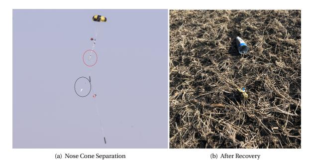
Figure 88: Successful Nose Cone Deployment
