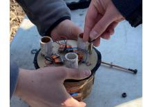
Figure 113: Inserting the Bolts to Connect Bulkhead to CRAM Body
