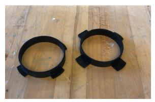
Figure 125: Sub-scale drag tabs
