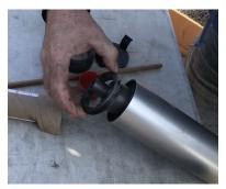
Figure 104: Addition of the Retaining Ring to the Forward Enclosure End of the Motor Casing
