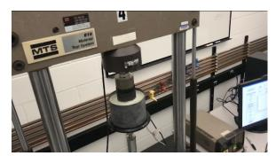
Figure 122: Centering Ring System in Test Machine
