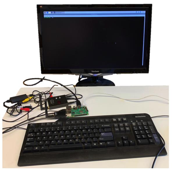
Figure 75: Primary ground station Raspberry Pi and connected hardware.
