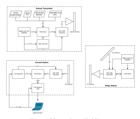
Figure 49: Telemetry System Block Diagram
