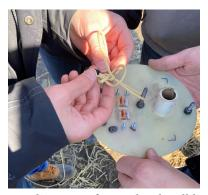
Figure 117: Bowline Knot for Payload Bulkhead Eyebolt
