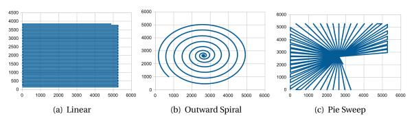
Figure 72: Simulated Flight Paths
