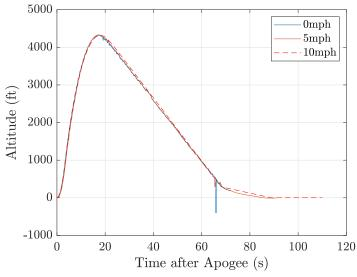
Figure 95: Updated Simulation compared to payload verification flight
