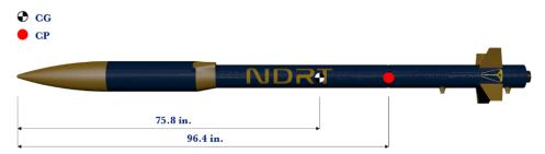
Figure 53: Simulated Loaded Static Stability Margin
