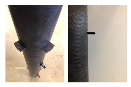
Figure 30: Drag Tab Deployment Through Fin Can Slots
