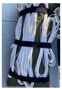
Figure 110: The Z-Folded Shroud Lines in Parachute Bag
