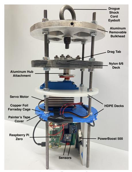
Figure 17: Fully Constructed ABS
