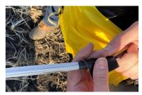
Figure 108: Taping the Shroud Lines to Ensure They are Straight
