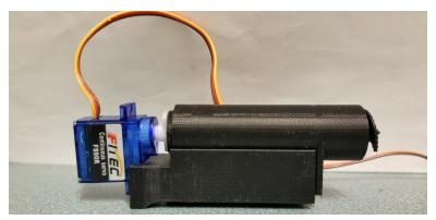
Figure 85: Assembled Sample Retrieval Screw
