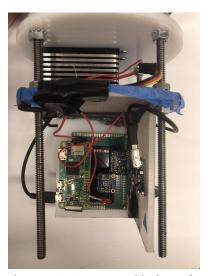
Figure 28: Electronics integrated below aft HDPE deck
