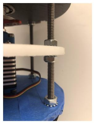
Figure 27: Lock nuts securing HDPE deck to threaded rods
