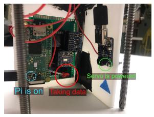
Figure 107: The LED Layout for ABS Functionality Confirmation
