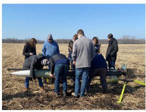
Figure 106: Lowering the Rail and Aligning the Rail Buttons
