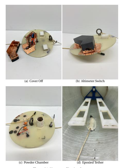
Figure 64: Nosecone Ejection System
