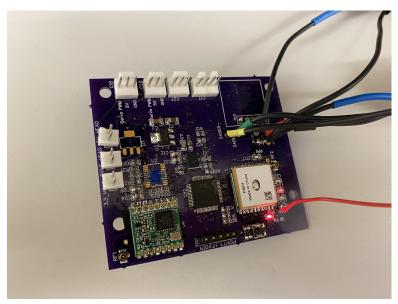
Figure 83: Rover Custom Circuit Board
