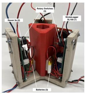
Figure 45: Assembled and Labelled CRAM Core
