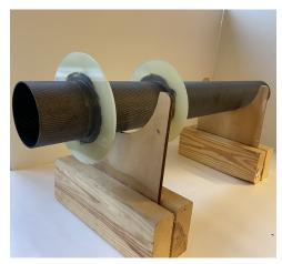
Figure 15: Centering Rings Epoxied to Motor Mount
