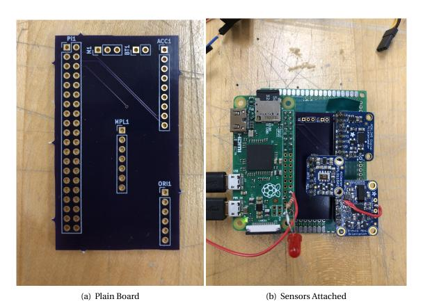
Figure 32: Printed Circuit Board
