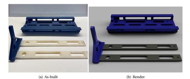
Figure 58: Sliding and Rail platforms
