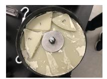
Figure 121: Angled Bulkhead with Supports Failure
