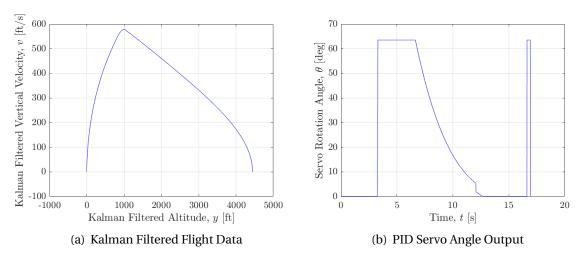
Figure 128: Control Structure Simulated Flight Test Data
