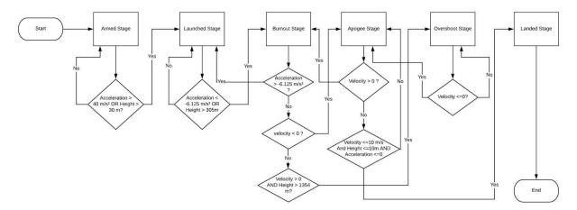
Figure 33: Updated Flow Chart of ABS Control Stages
