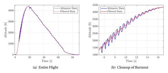
Figure 34: Raw and Filtered Altitude Data
