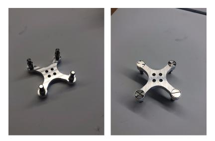
Figure 23: Upper Piece of the Aluminum Crosspiece with Press-fit Shoulder Screws
