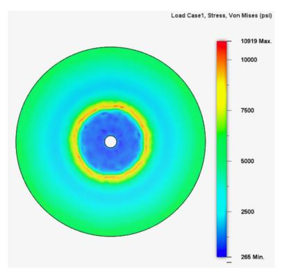
Figure 11: FEA on Payload Bulkhead (von Mises Stress)
