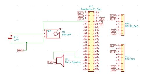
Figure 31: Schematic of Final Electronics Wiring
