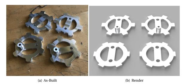
Figure 78: Aluminum Hubs
