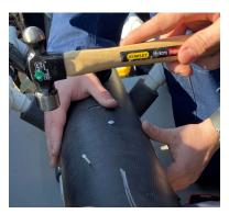
Figure 100: Securing the Fin Can to Recovery Tube with Shear Pins
