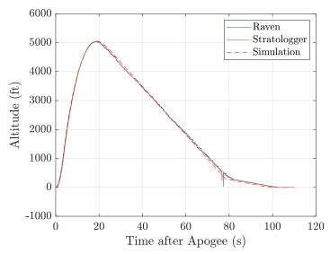
Figure 93: Updated simulation compared to vehicle demonstration flights
