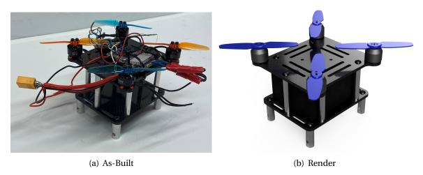
Figure 67: UAV Assembly
