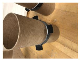
Figure 126: Sub-scale drag tabs on coupler
