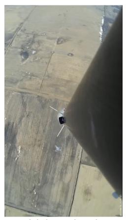
Figure 129: Drag tab deployment during demonstration flight
