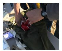
Figure 112: The Folded Drogue Being Folded in the Nomex
