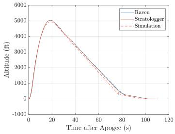
Figure 92: Simulation compared to vehicle demonstration flight
