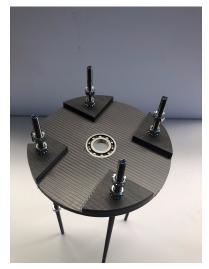
Figure 21: Nylon 6/6 Slotted Deck with Press-fit Ball Bearing
