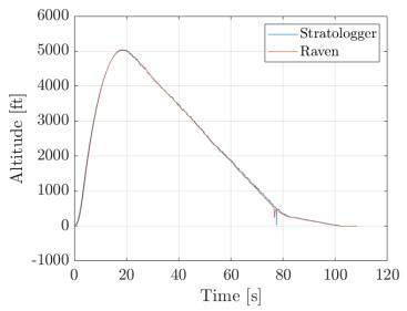
Figure 91: Flight profile data for vehicle demonstration flight
