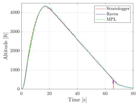
Figure 130: ABS MPL3115 altitude data compared to recovery altimeter data
