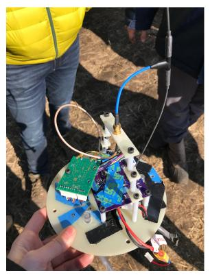
Figure 52: Fully assembled flight configuration of telemetry system and telemetry bulkhead
