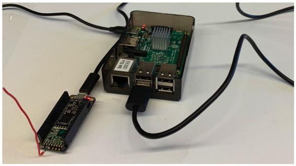
Figure 76: Rover Control Module Raspberry Pi and connected hardware
