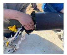
Figure 98: Packing the Parachute Below the Transition Section
