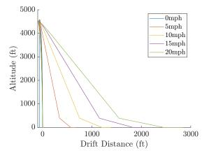
Figure 55: Predicted drift for various launch conditions
