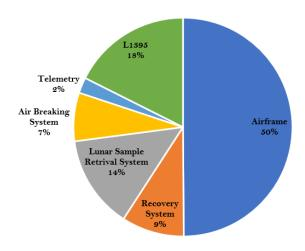
Figure 3: As Built Mass Breakdown
