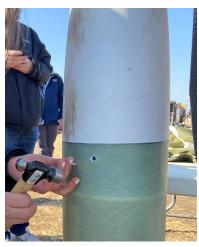
Figure 101: Insertion of Shear Pins in Nose Cone
