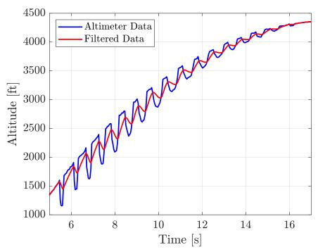
Figure 131: Close-up showing drops in the altitude data
