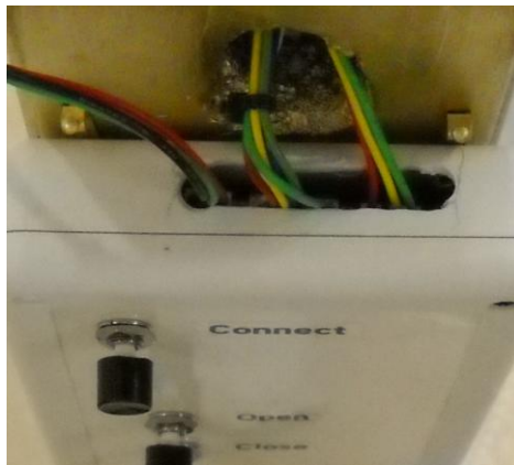
Figure 4.1.2d Port placement on the top of the window control box. From left to right: light sensor, window assembly connector, motor connector.
