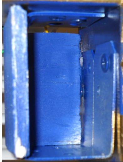
Figure 4.1.2b Proper installation on the battery mounting brackets.
