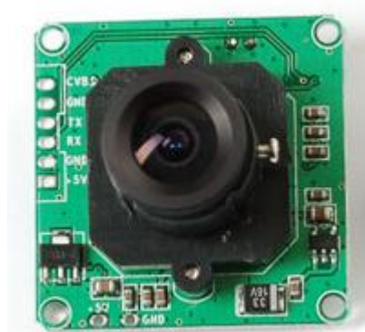
Figure 3.7.1. Adafruit TTL Serial JPEG Camera ( https://www.adafruit.com/products/397 )
