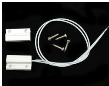
Figure 3.3.1. Magnetic Contact Switch ( https://www.adafruit.com/products/375 )
