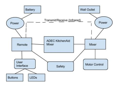
This block diagram above displays the various subsystems for the mixer. The system is split into two different devices: the mixer itself and the remote control. They are connected by an infrared transmitter and receiver. Both devices have a power component. The remote has a user interface component including buttons for speed selection and lights and icons to show various things to the user.
