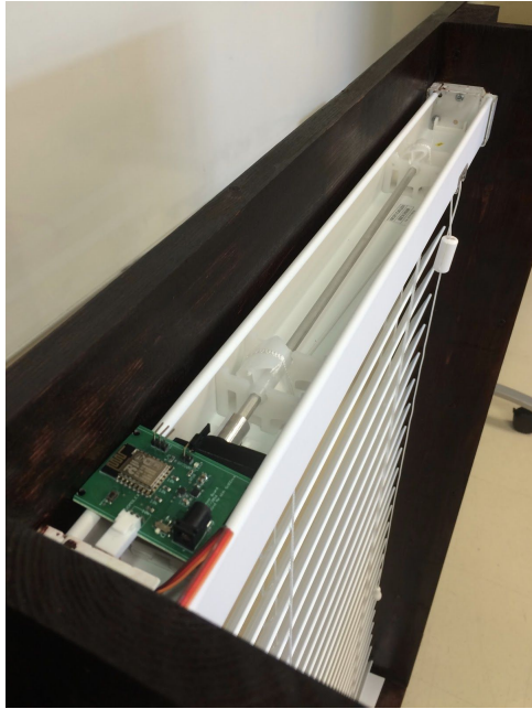
Figure 8. Servo and Blinds Mechanical System
