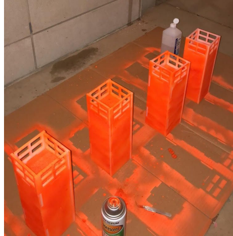
Figure 3-15: Left to right: completed construction of pylons (without platforms), final construction with platforms inserted and painted to mimic football pylons.
