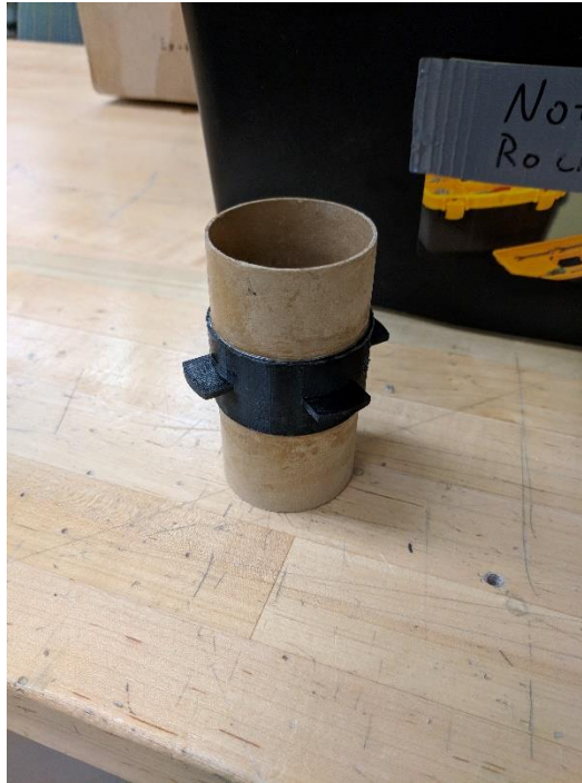
Figure 75. Image of the tab coupler used in the subscale flight test.
