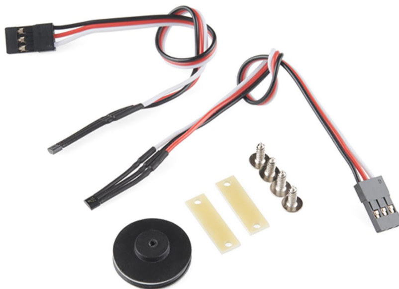
Figure 45. Wheel Encoder Kits from DAGU will be used with the Turnigy motors.
