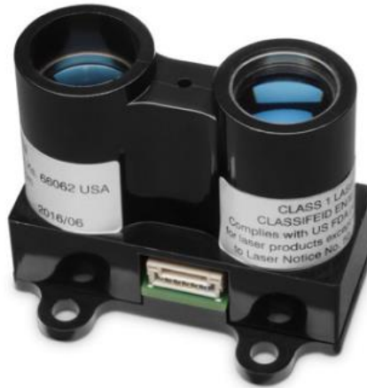
Figure 58. A Garmin LiDAR Lite v3, SEN-14032 will be used for object avoidance.
