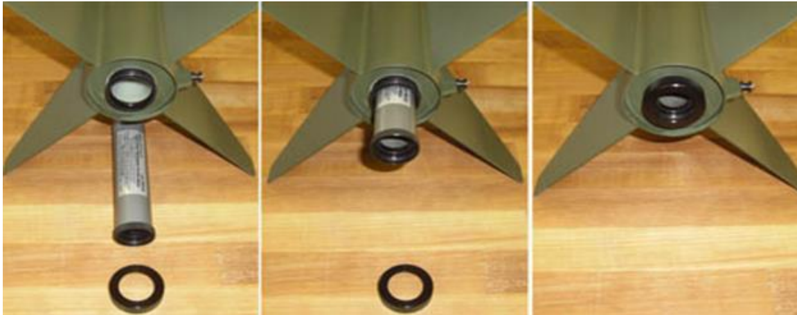
Figure 17. Cesaroni Pro29 motor assembly using 29 mm Aero Pack Quick-Change motor retainer system.
