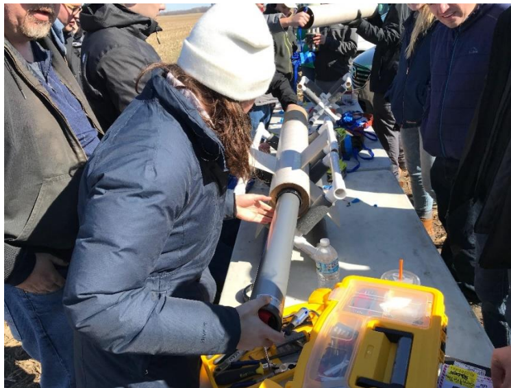
Figure 25. Cesaroni 75 mm Motor Casing being inserted into rocket.
