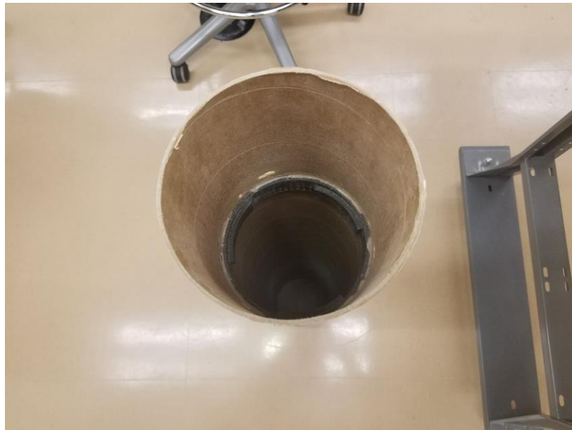
Figure 41. The mount (black) shown securely epoxied within the phenolic recovery body tube.
