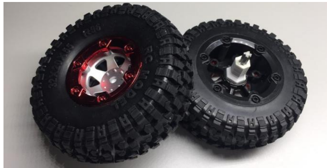
Figure 65. Custom 3D printed hubs provide a secure connection between the wheels and motors.
