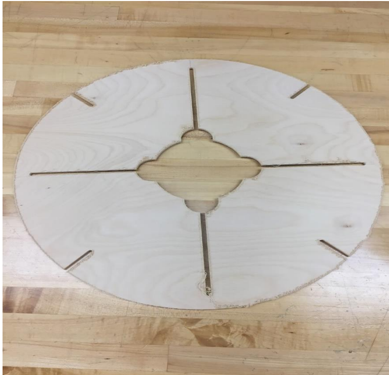
Figure 36. Laser cut Fin Alignment Mechanism.
