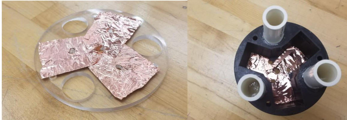
Figure 55. Copper shielding above and beneath avionics.
