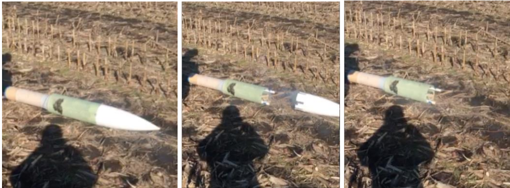
Figure 127. Screen grabs from the video of the black powder and deployment test of the rover payload.
