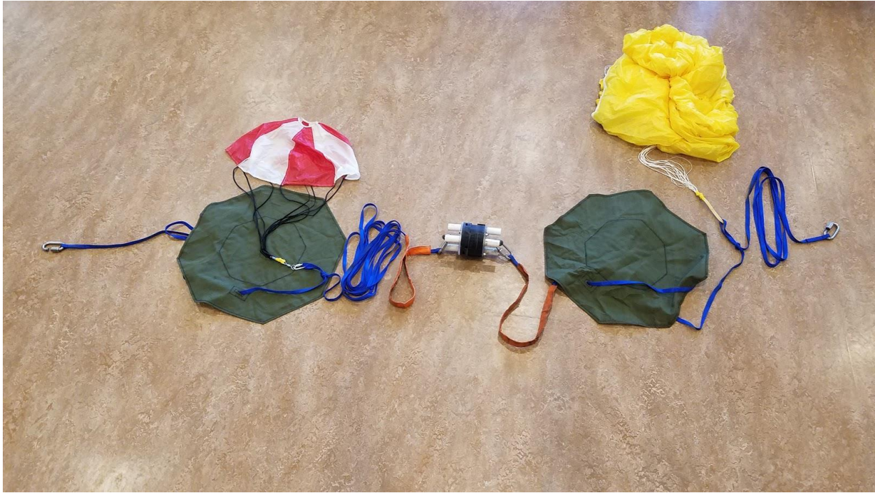
Figure 46. Assembled recovery system.
