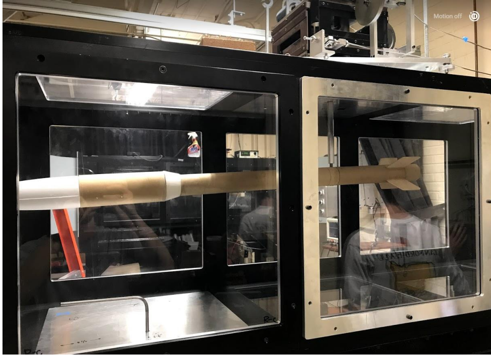
Figure 56. Wind tunnel test setup.
