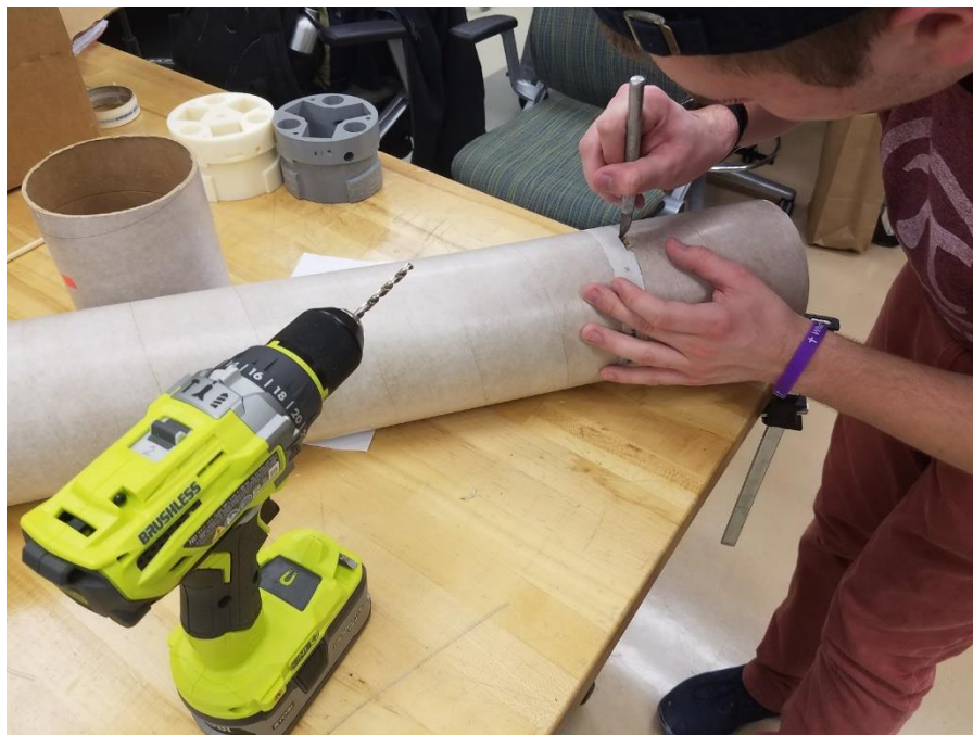
Figure 33. Cutting Slots for the Recovery System.
