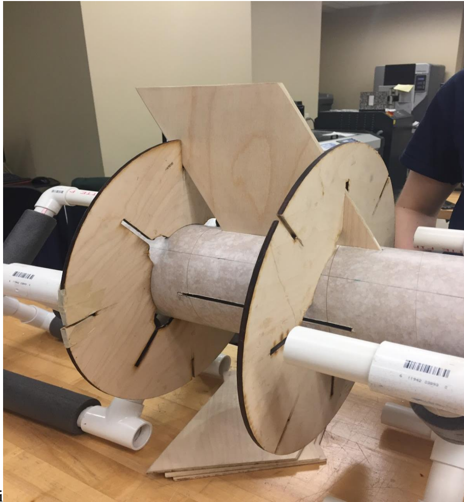
Figure 34. Fin Insertion Process.
