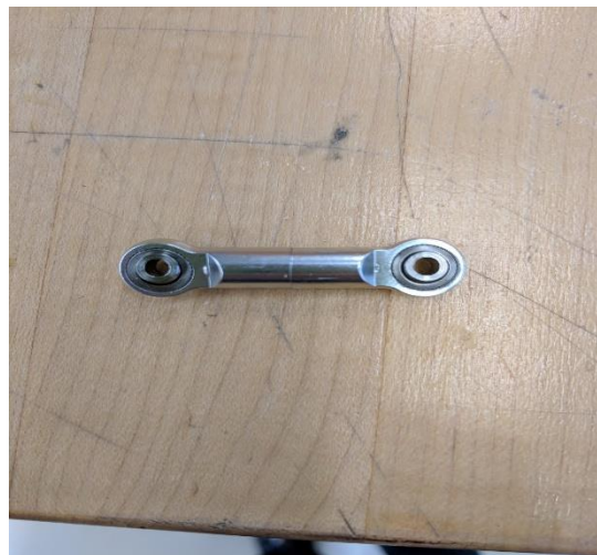
Figure 98. A detailed drawing and picture of one tie rod, though there are four on the real mechanism. Units in inches.
