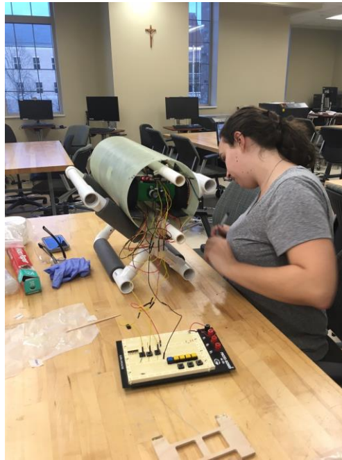
Figure 125. The actuation of the racks into the securing mount was tested to ensure the alignment of the mounts match the alignment of the solar panel racks. This also tested the servomotor's dual functionality as the securing system.
