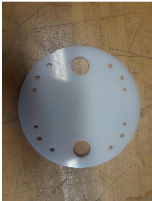
Figure 116. Battery deck without components attached.
