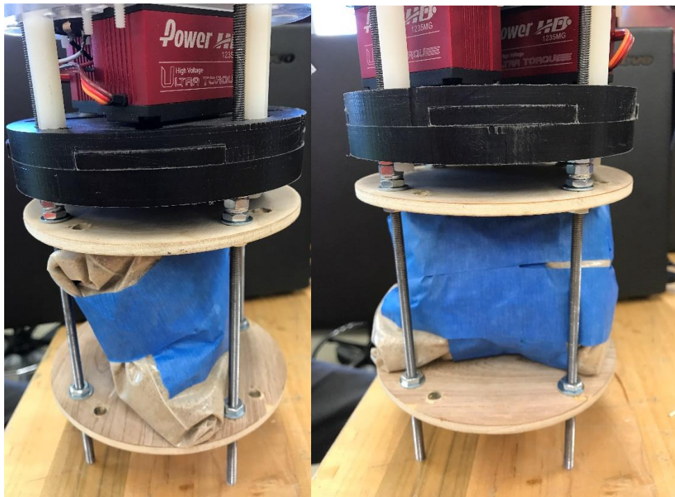
Figure 27. Ballast between couplers of the Air Braking System.
