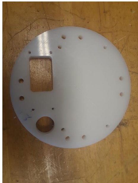
Figure 115. Microcontroller deck without components attached.
