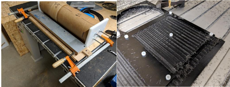
Figure 102. Router securing fixtures for the tab sheet and payload coupler.
