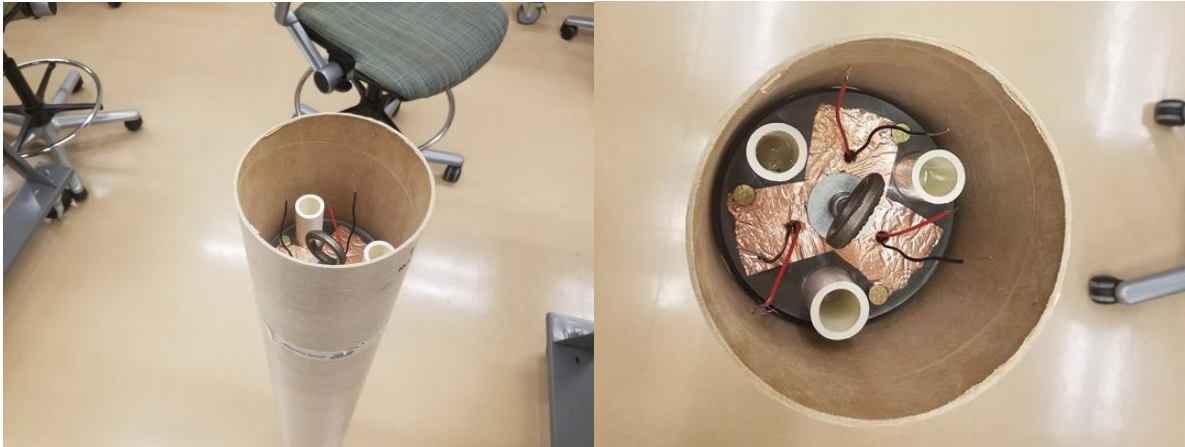
Figure 45. CRAM v4, inserted into the recovery body tube.
