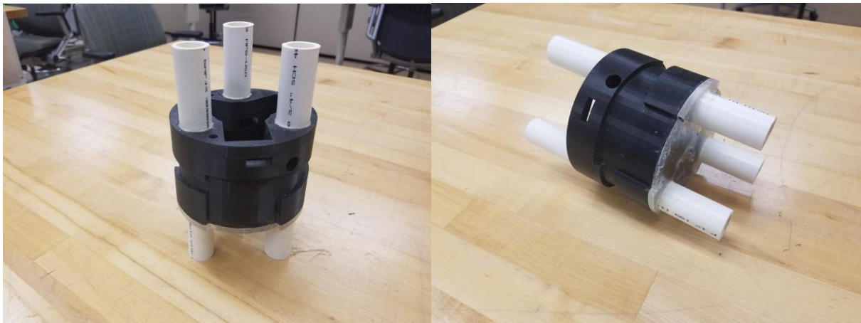
Figure 39. The CRAM body (black) with PVC pipes epoxied into place
