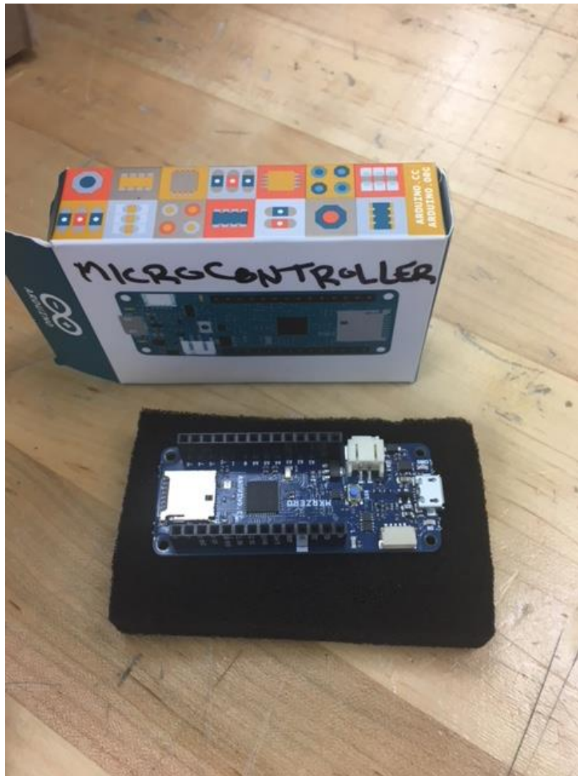
Figure 104. Image of the Arduino MKR Zero before integration into the system.
