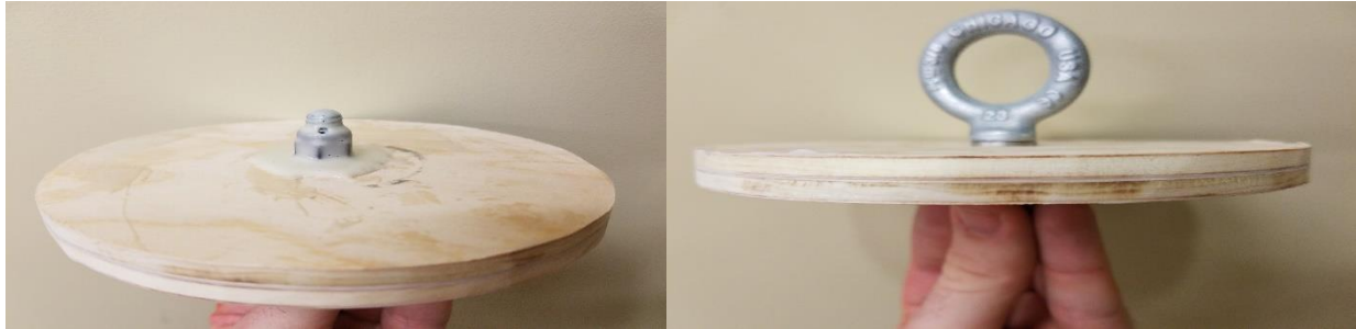
Figure 20. A plywood bulkhead used for recovery integration.
