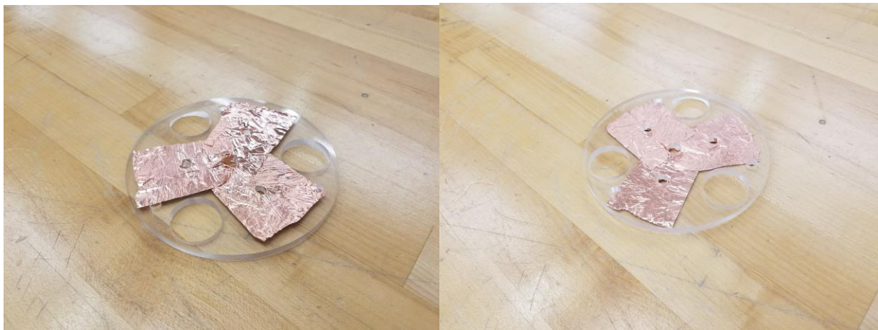
Figure 42. Top recovery bulkhead with adhered copper shielding.
