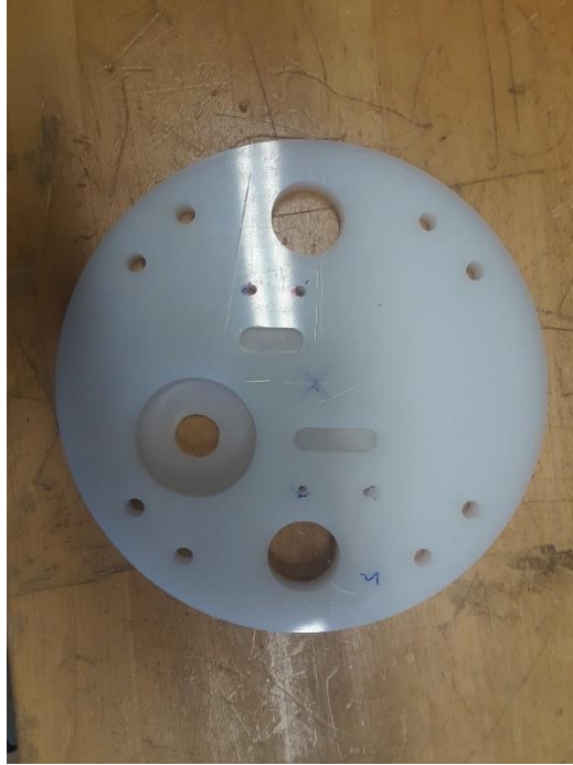
Figure 114. Sensor deck without components attached.
