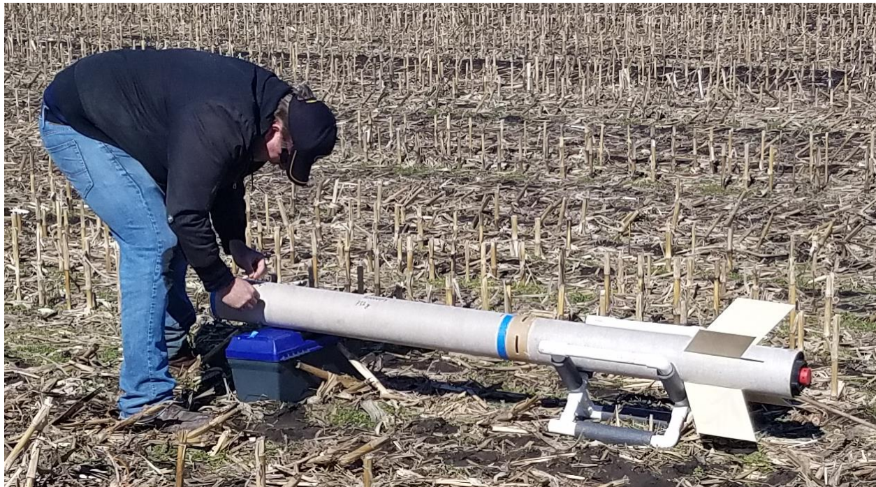
Figure 124. Black powder/shear pin ground testing.
