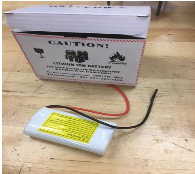
Figure 107. Tenery battery used to power the servo motors.
