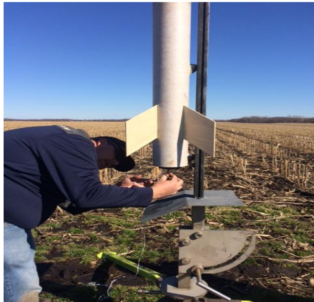
Figure 26. Michiana Rocketry Mentor inserting electrical igniter into motor on launch pad.
