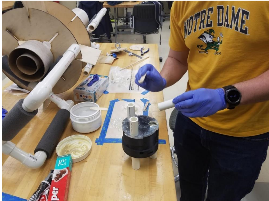
Figure 31. Attaching the PVC Pipe to the CRAM.
