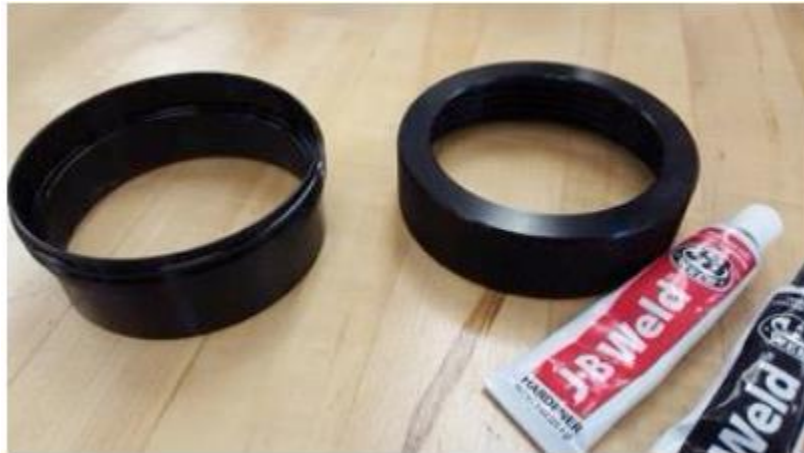
Figure 23. Pre-installed API Quick-Change 75 mm motor retention system.
