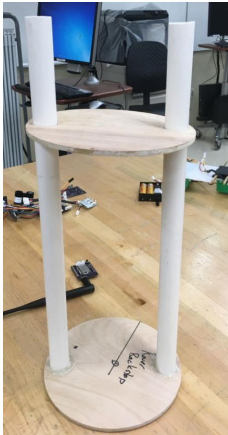
Figure 87. Mounting the PVC pipes to the back bulkhead.
