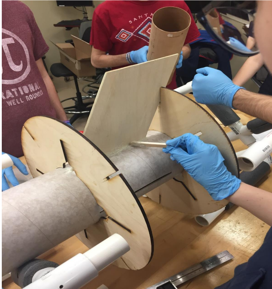
Figure 38. Fin Epoxying Process.
