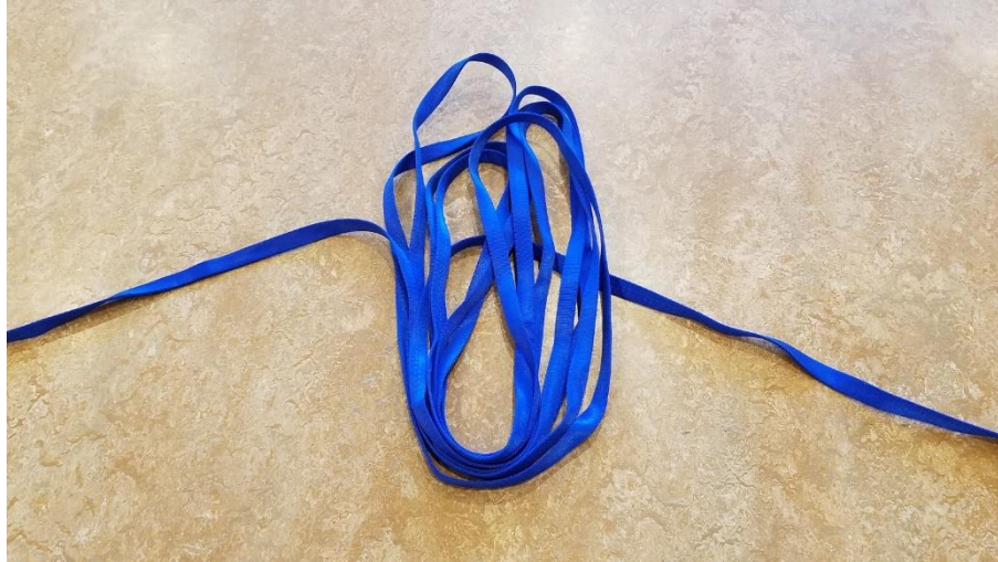
Figure 43. Shock cord used in the recovery system.
