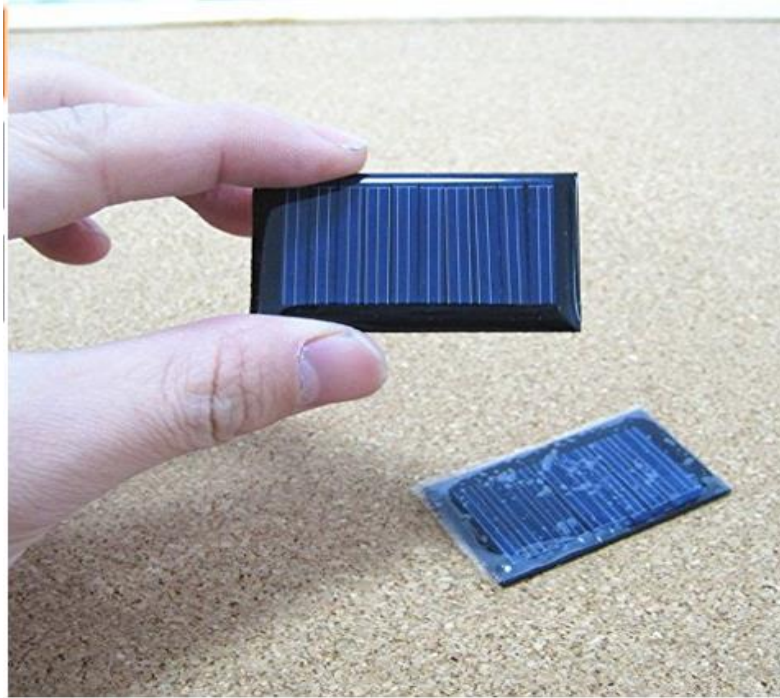
Figure 27. The solar panel structure will be constructed out of multiple small panels shown above.
