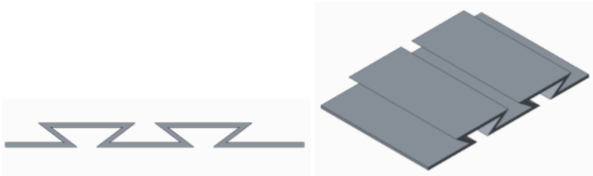
Figure 26. CAD rendering of the solar panel folding mechanism.
