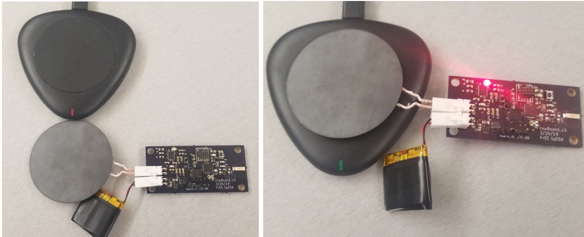
Figure 6: Board before (left) and during (right) wireless charging
