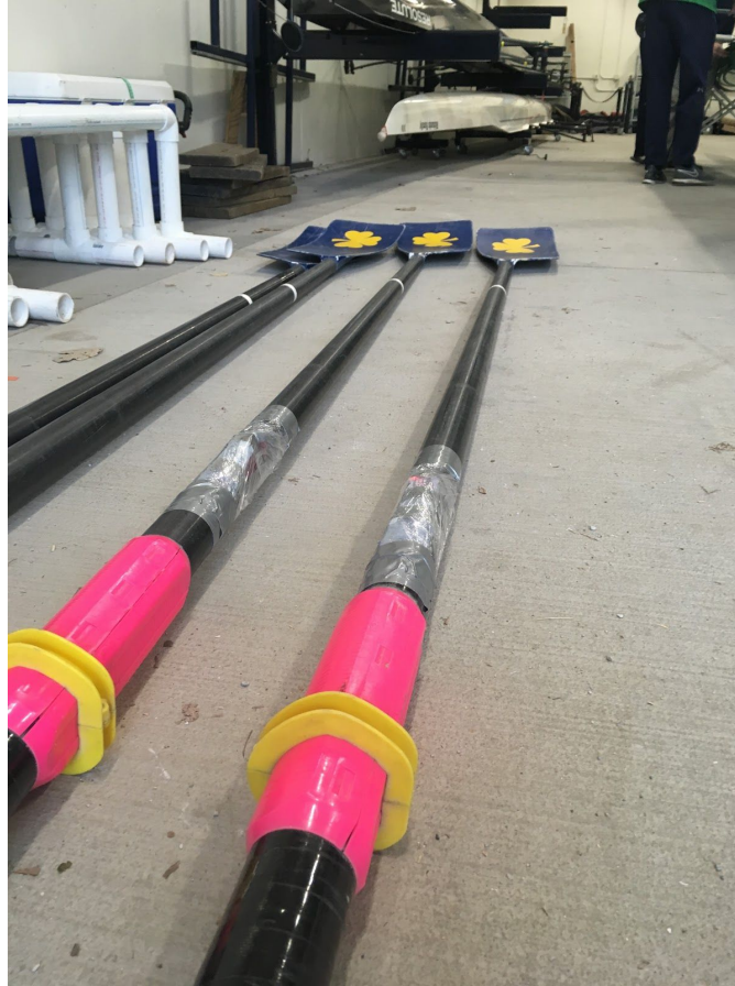
Figure 7: OarTracker device mounted on oars.
