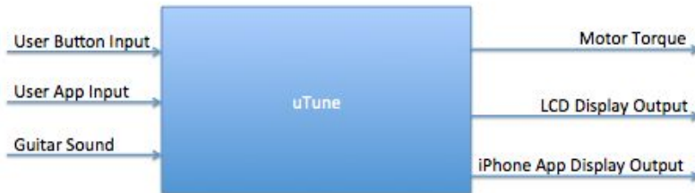
Fig. 1 - uTune "Black Box" Inputs and Outputs
