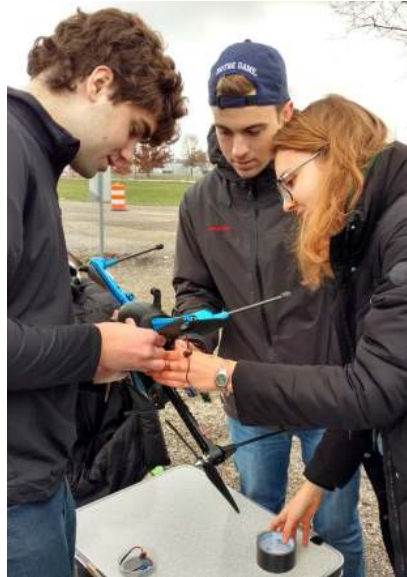
Figure 101: Team attaching the Raspberry Pi and its camera to the 3DR IRIS+ Quadcopter.
