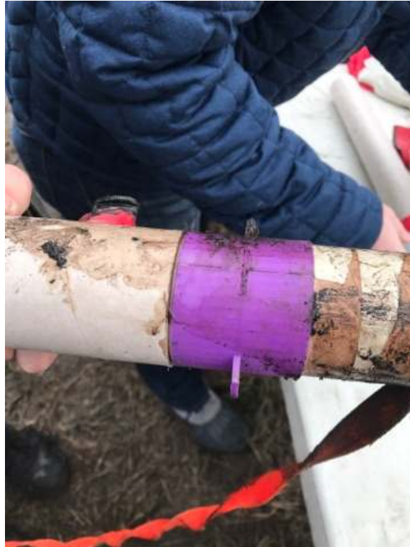
Figure 107: Subscale Drag Tab Coupler Upon Landing
