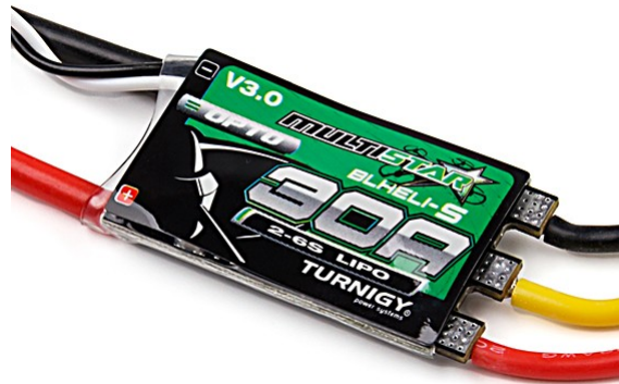
Figure 15: Electronic Speed Controller to reside on on UAV board.
