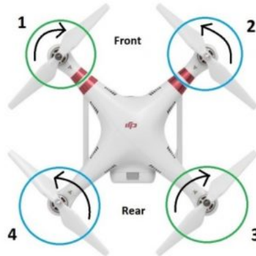
Figure 19: "X-configuration" for quadcopter design.
