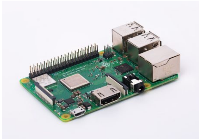
Figure 12: Raspberry Pi to reside on UAV board.
