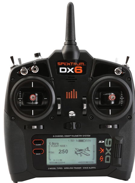
Figure 16: Transmitter to manually control the UAV.
