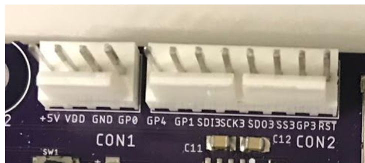
Figure 11. MOLEX Connectors For Communicating with Transceiver Board
