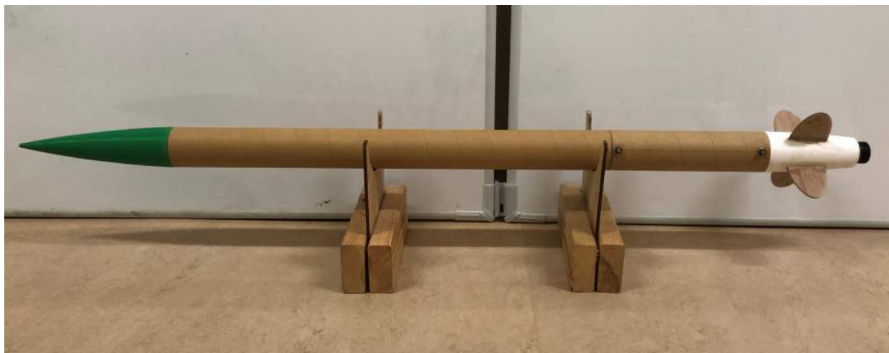
Figure 22: Image of the fully constructed subscale launch vehicle
