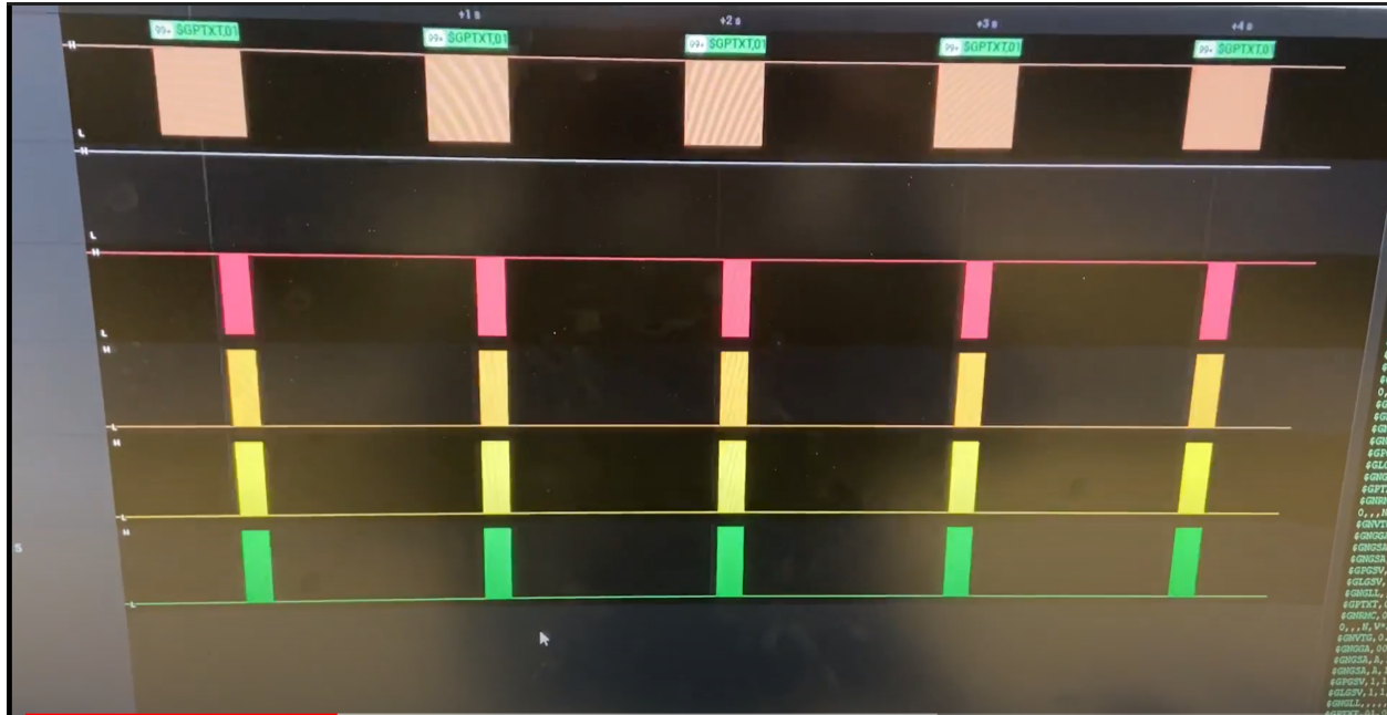
Figure 1. Logic Analyzer Output on UART and SPI communications for Balloon subsystem sending GPS Data
