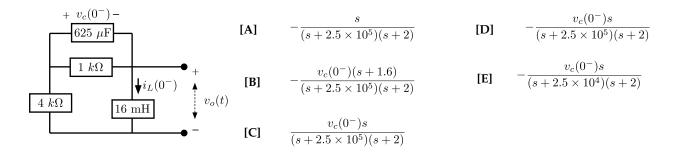
Multiple Choice Question 6: Consider the circuit shown below. Assume there is no energy stored in in its inductors and capacitors just before time t = 0. Determine the single sided Laplace transform of the voltage waveform  $v_o(t)$ .
