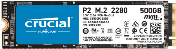
Solid State Drive (Crucial CT500P2SSD8)
