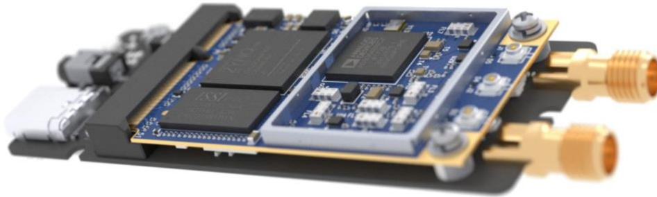
Figure 19. Sidekiq Z2 software-defined-radio
