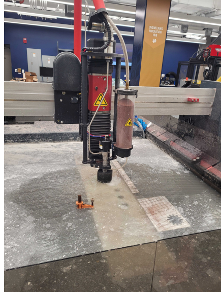
Figure 25: Water Jet Cutting Submerged G10 Fiberglass Sheet
