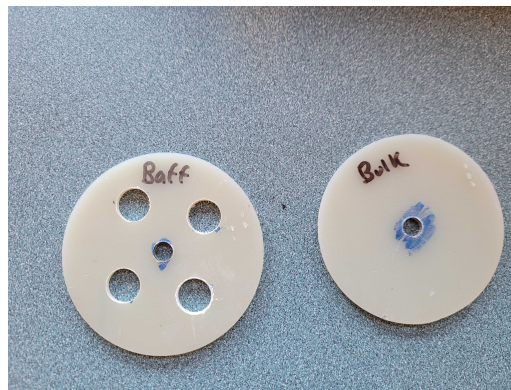
Figure 26: Baffle and bulkhead
