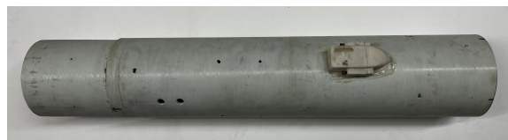
Figure 26: Constructed Payload Bay
