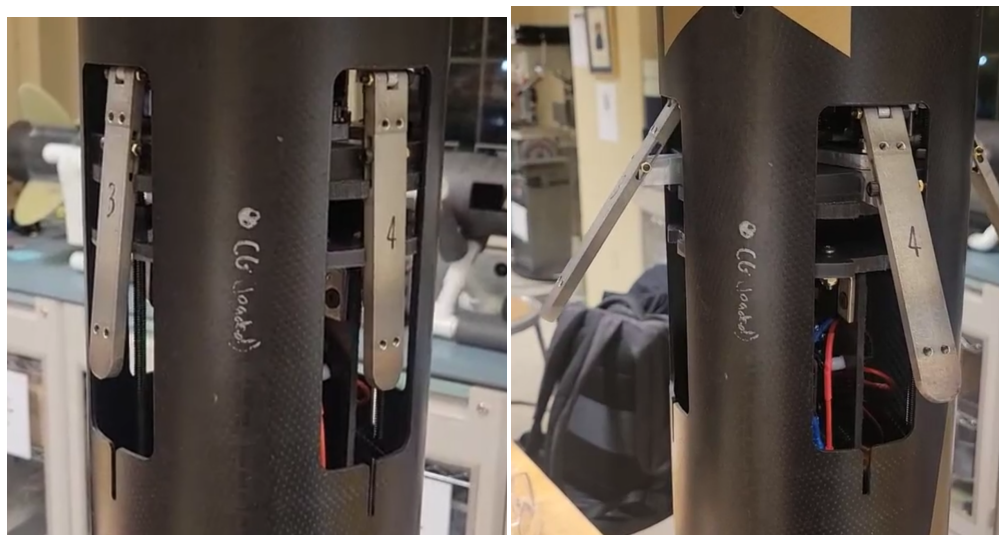
(a) Drag flap retention
