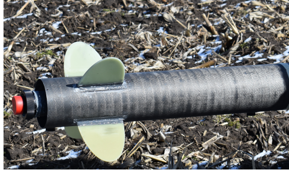
Figure 30: Constructed Fin Can
