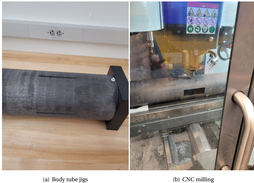
Figure 17: Cutting ACS Flaps and Fin Slots
