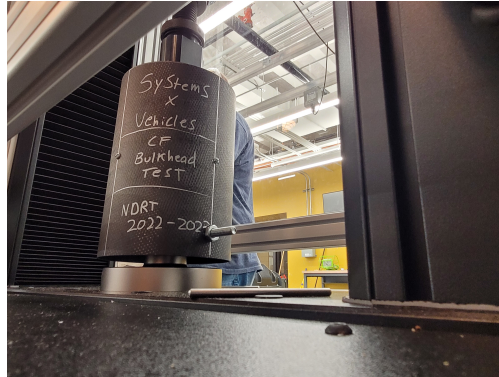
Figure 124: Bulkhead static loading test setup
