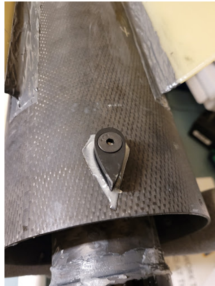
Figure 21: Rail Buttons Epoxied to Fin Can
