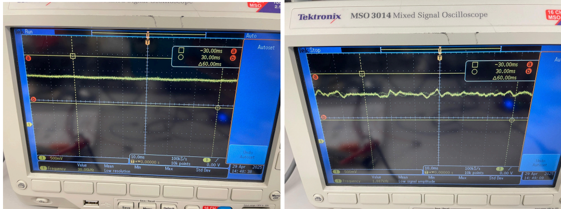
Figure 6. Relaxed vs. Flexed Signal at Output of Instrumentation Amplifier
